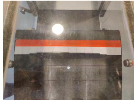
(b) *The large airfoil (198 mm chord length) at a 13° angle of attack*
