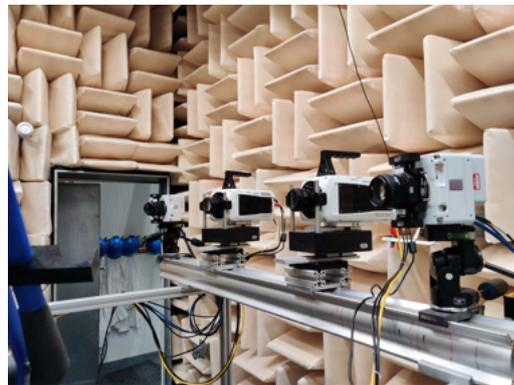
(b) *The four Phantom slow motion cameras used for capturing the data.*
