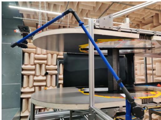
(a) *The arm with laser optics of the illumination system.*
