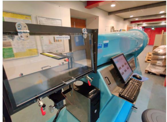
Figure 9: Image of the setup with the 3D printed airfoil on the stinger balance of the small wind tunnel with one of the laser cut flaps installed.
