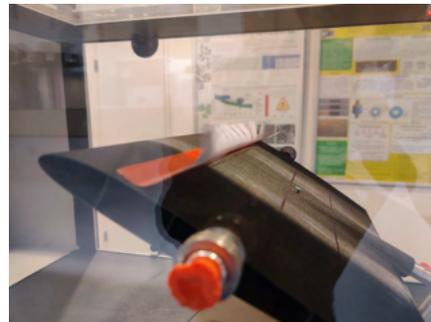
(b) *The large airfoil (198 mm chord length) at a 27° angle of attack*
