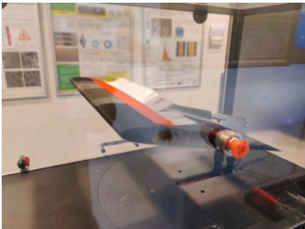
(a) *The large airfoil (198 mm chord length) at a 13° angle of attack*
