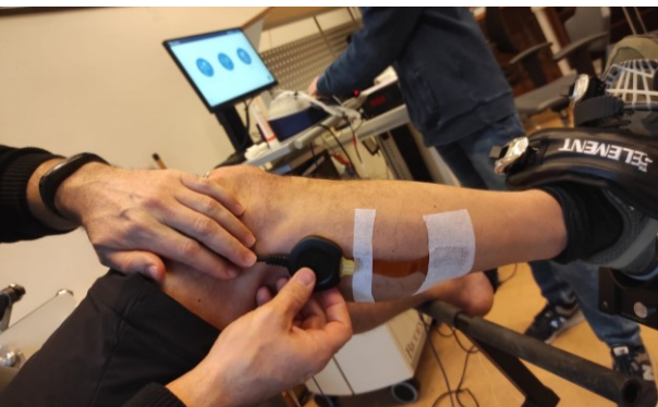
Fig. 9. Positioning of a semi-disposable 64-channel electrode and reference electrode during experimentation.
