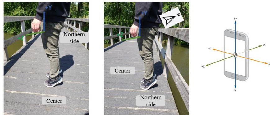
Figure 19 - Load cases 2&3: heel drop at the center (case 2) and at the northern side (case 3), and smartphone measurement directions
