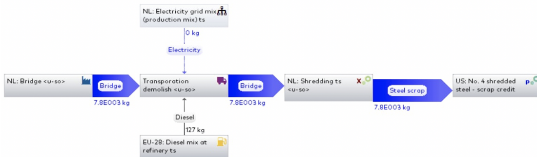
FIGURE 28: Disposal process, 3D printed bridge
