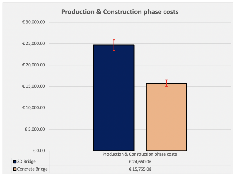
FIGURE 53: Histogram Production-Construction phase costs
