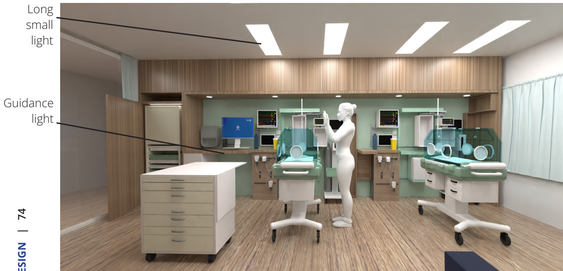
Figure 46, Final lights design for the single room unit shown from the front of the incubator
