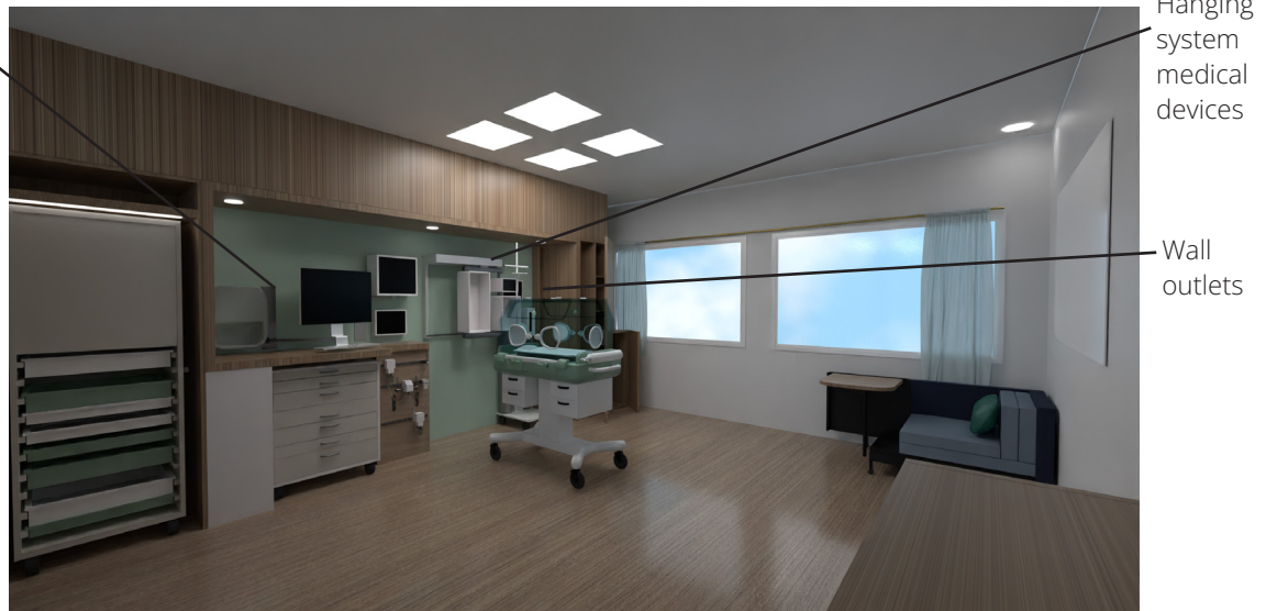
Figure 34, Second iteration design for the single room unit facilitating one baby shown from the left side of the incubator
