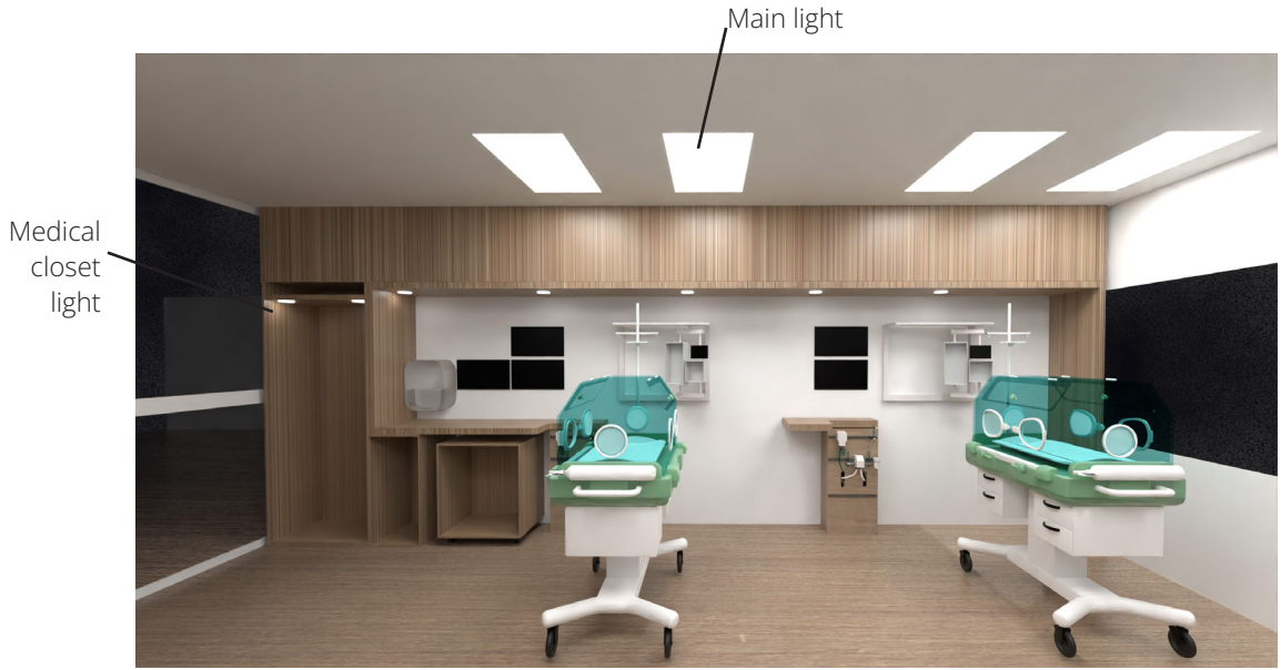
Figure 29, First iteration of the lights design for the Single Unit room shown from the front of the incubator
