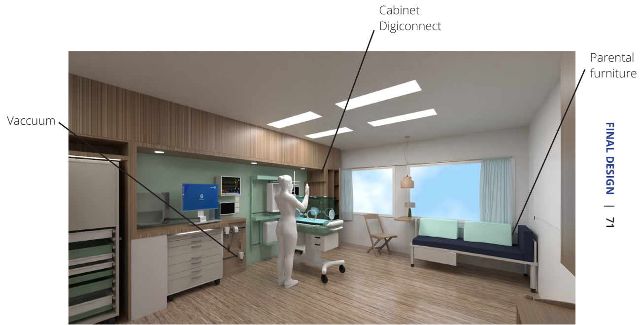
Figure 42, Final design for the single room unit facilitating one baby shown from the left side of the incubator
