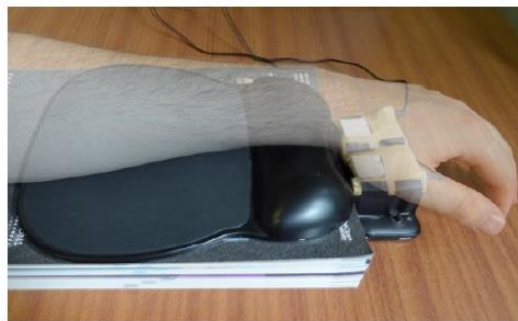
Figure 6 - Experimental setup of Wilson, Davidson & Brewster with Peltier elements under the palm and the padded armrest for comfort [27]
