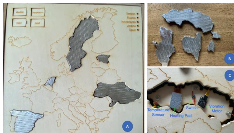
Figure 5 - (A) The physicalisation that uses temperature ( T ) and vibration ( V ) to represent Affordable and Clean Energy data of five countries: Sweden, Estonia, The Netherlands, Ukraine and Spain; (B) Laser cut wooden buttons (representing the geometric shape of the country) wrapped in metal to enable heat conductance; (C) Internal organization (using Sweden as example) of electronics and sensors to enable vibration and temperature output [10].
