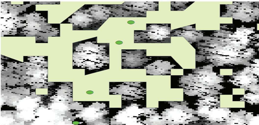
Fig. 2.9 . Problem of interconnected gaps with automatic delineation. The green points represent coordinates of gaps sampled in field. They have been detected correctly, however, due to a narrow passage of pixels with low vegetation; they are connected, which makes it almost impossible to calculate the area of one single gap.
