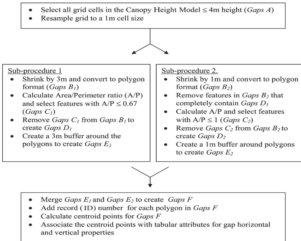
Fig 2.4. Summary Procedure for gap delineation, (Corresponding & Blackburn, 2004).
