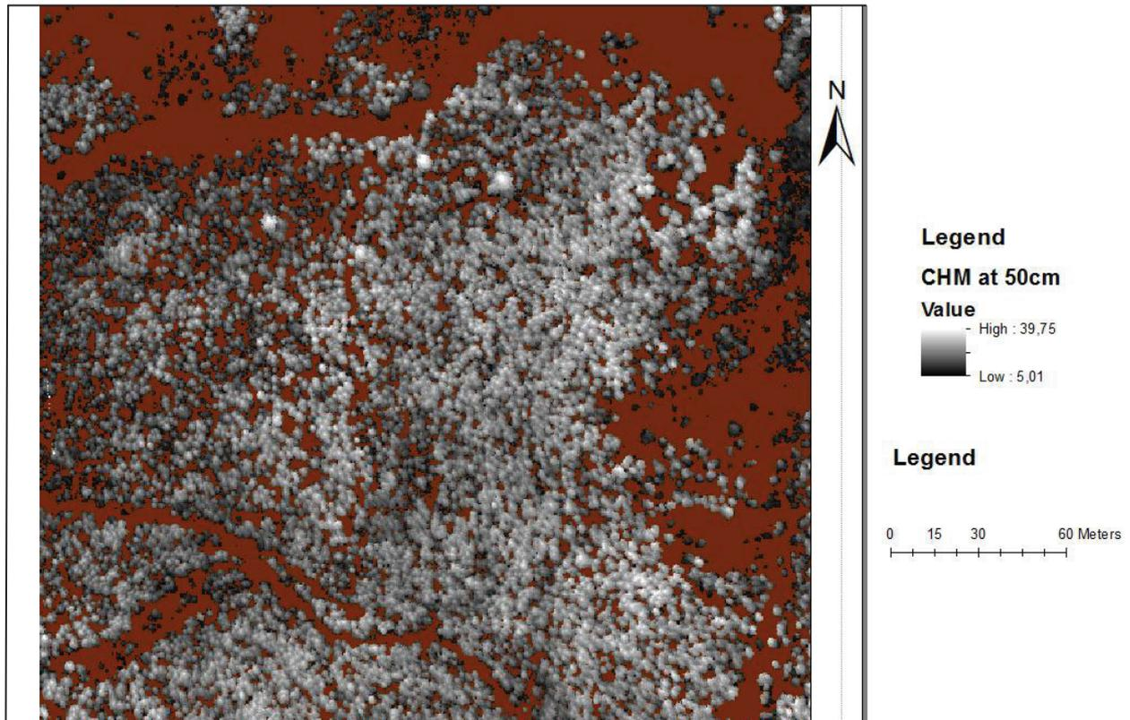
Fig.3.5. Canopy Height Model at 50cm. All the pixels with a value below 5 have been assigned as 'nodata'.
