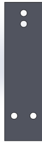
Figure 37: Laser cut plexiglass in between which the SMP get clamped. The two plexiglass plates get secured on the sliding elements at the top and the SMP will be clamped at the bottom.
