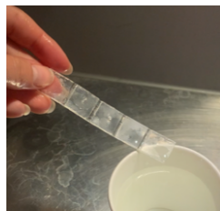
Figure 11: A five panel SMP with laser cut hinges.
