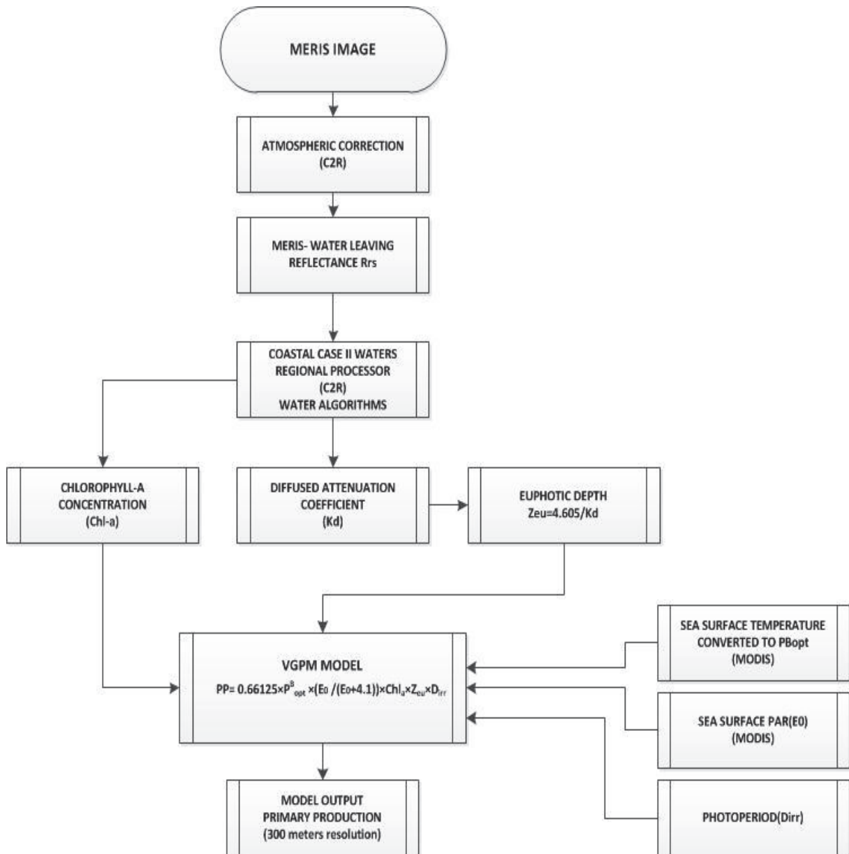
Figure 4.1 Model schematic representations of MERIS-MODIS images processing for primary production
