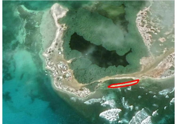
Figure 55, An overview of the current situation at Lac Cai were a pile of rocks is deposited perpendicular to the coast in the form of a breakwater (Google Earth)
