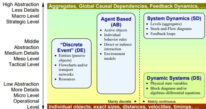
Figure 3.2: Overview of the different simulation types and the usage of each of the approaches within the different management levels (Borschev & Filippov, 2004)
