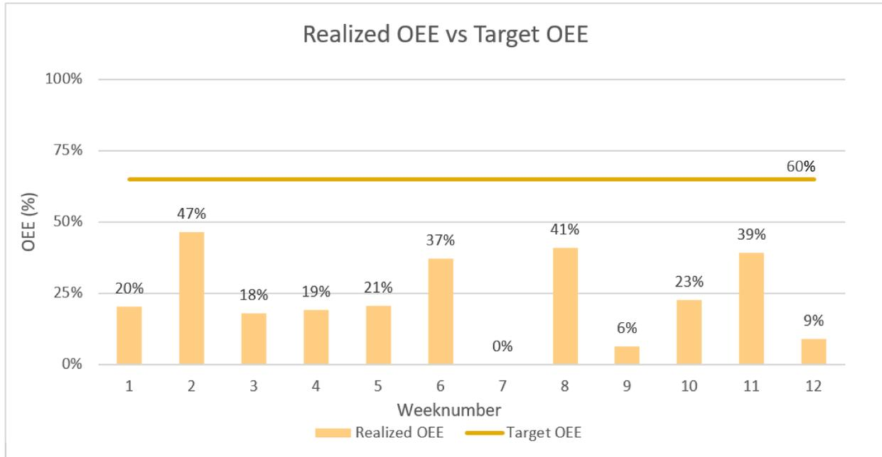
Figure 2.5: Development of the OEE Key Performance Indicator (KPI) for the palletizing robot during the first 13 weeks of 2022
