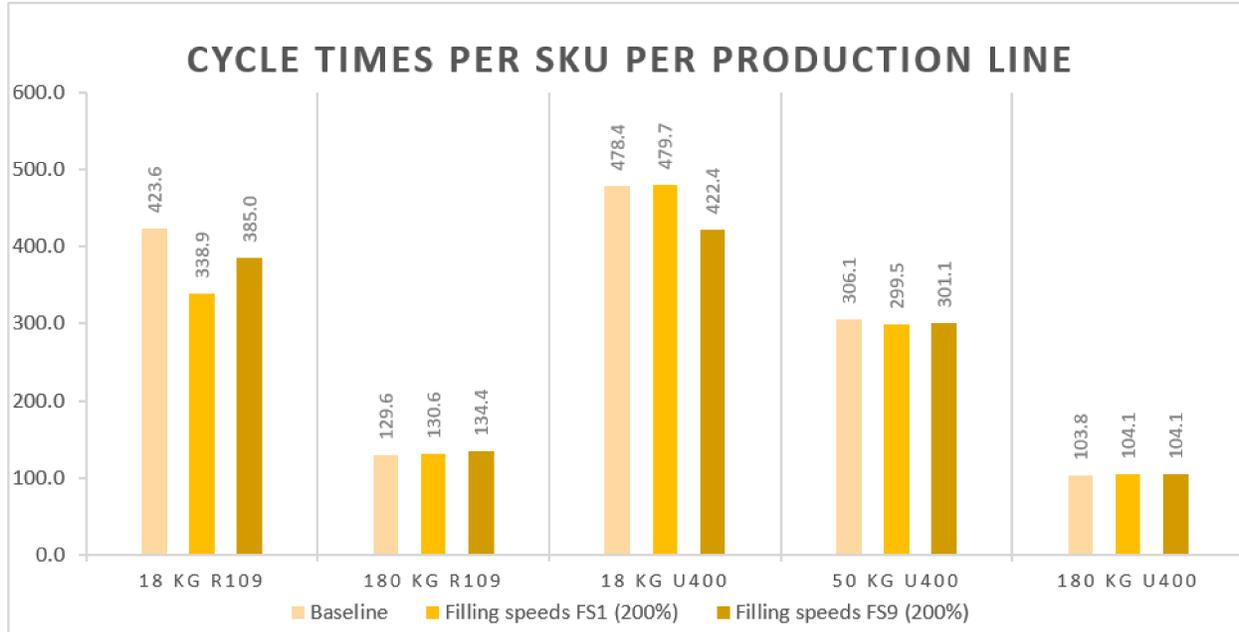
Figure 5.6: Results of the average cycle times per experiment 9 and 10 for the different SKUs filled at production lines R109 and U400
