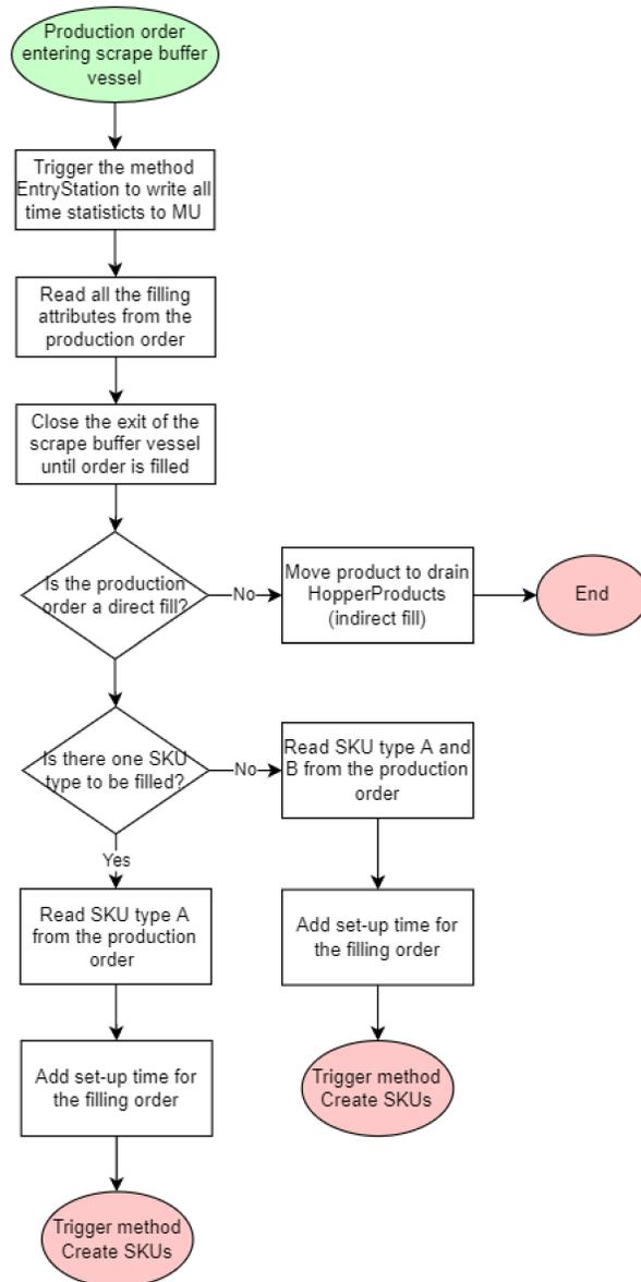
Figure 4.4: Flowchart of the production order entering the scrape buffer vessel after it has been processed on all three kettles. This holds for both the R109 and the U400 production lines.
