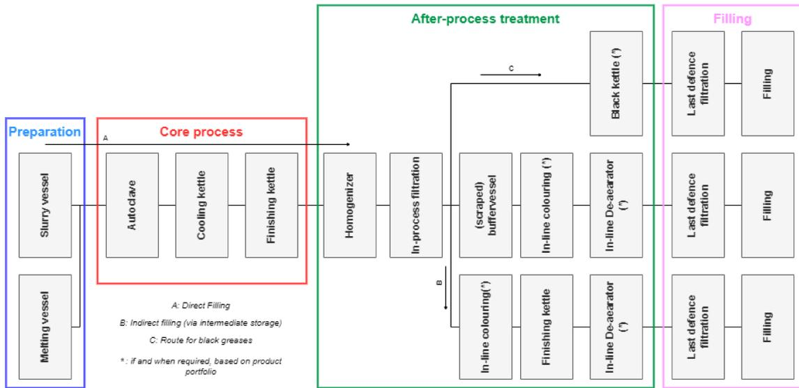
Figure 1.1: Global representation of Shell's production process within Ghent's GMP
