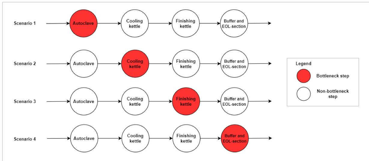
Figure 2.3: Overview of the bottlenecks in the production processes for both the R109 and the U400 production lines, with the red marked circles identifying the bottlenecks in the production process.
