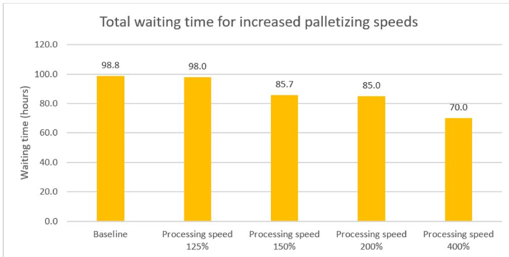
Figure 5.1: Overall waiting time for experiments 1-4 with an increased palletizing capacity
