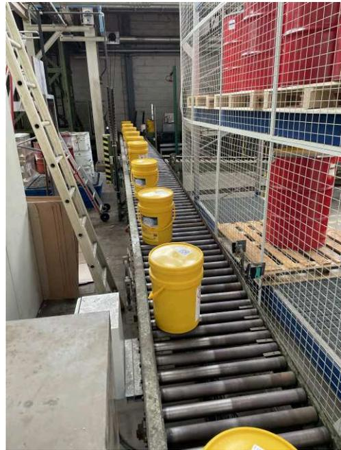
(b) Conveyor belts to the palletizing robot from FS9
