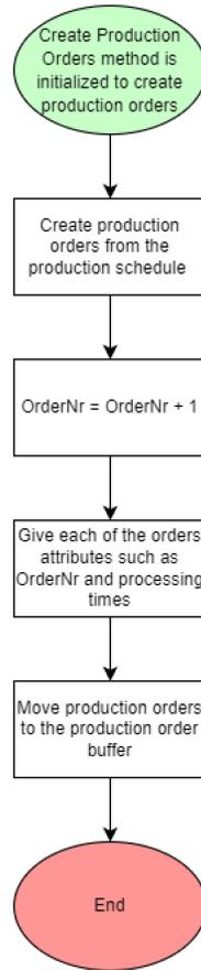
Figure 4.2: Flowchart of the initialization and creation of the production orders in the process. This logic holds for both the R109 and the U400 production lines.
