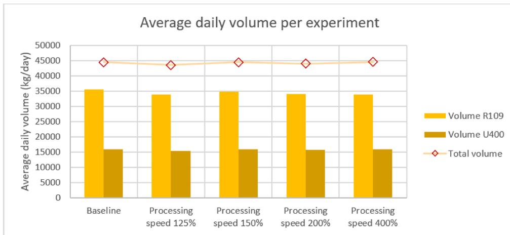
Figure J1: Average daily volume for experiments 1-4 with an increased palletizing capacity
