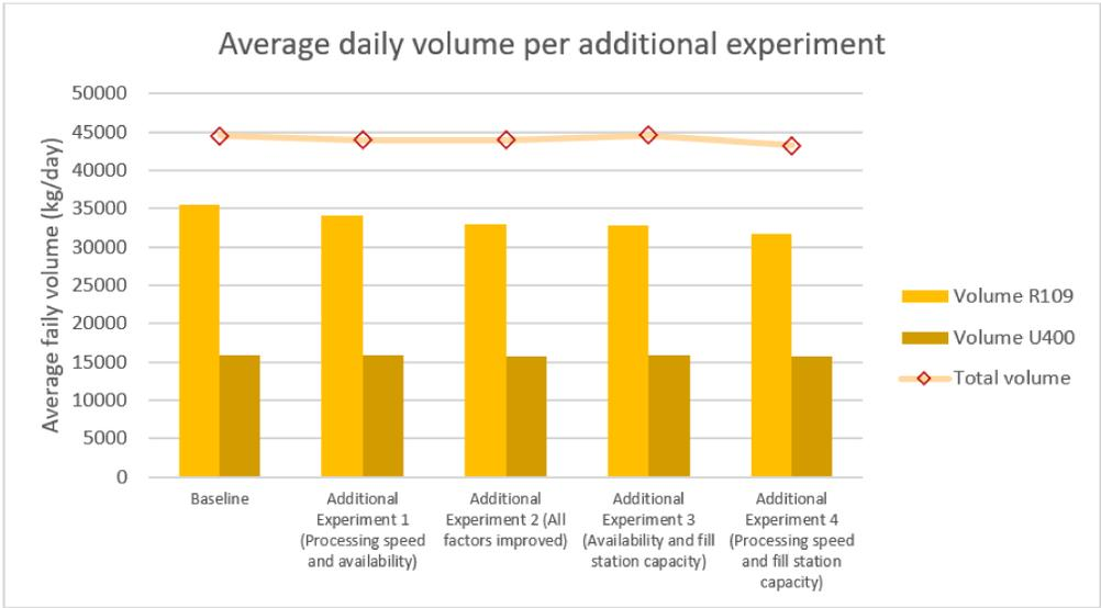
Figure J4: Average daily volume for experiments 9 and 10 with an increased palletizing capacity
