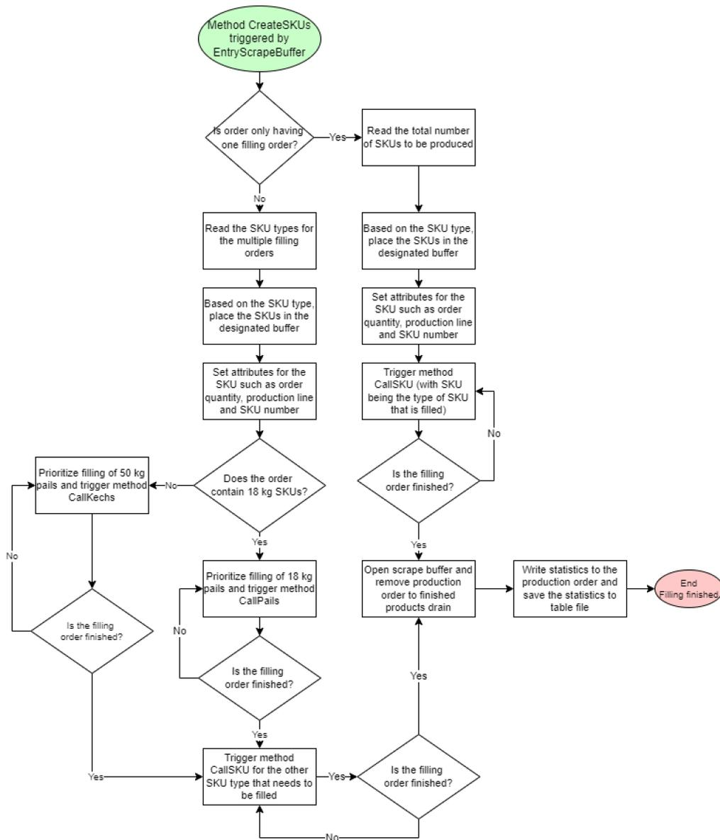
Figure 4.5: Flowchart of the creation of the SKUs after the production order has arrived in the scrape buffer vessel. This logic holds for both the R109 and the U400 production lines.
