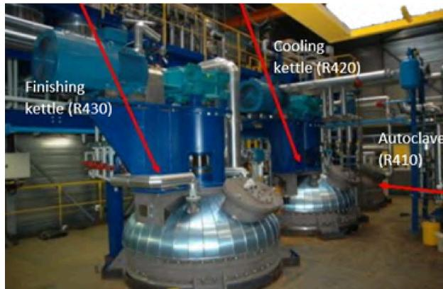
Figure A.2: U400 platform with from left to right the finishing kettle, cooling kettle and autoclave.
