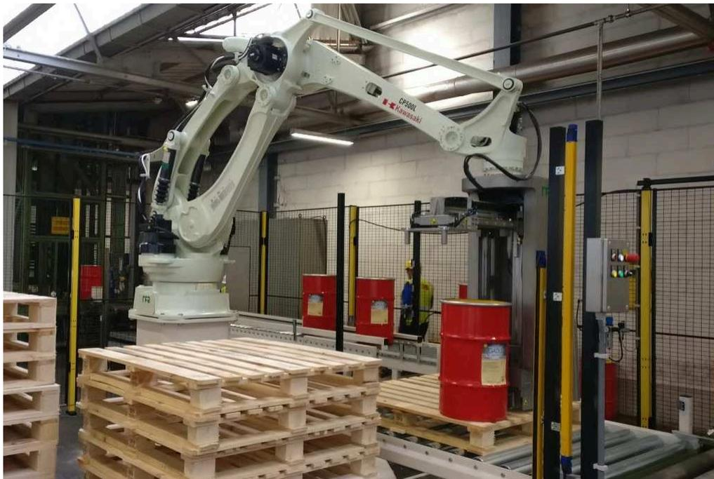
(c) Palletising robot at the EOL section
