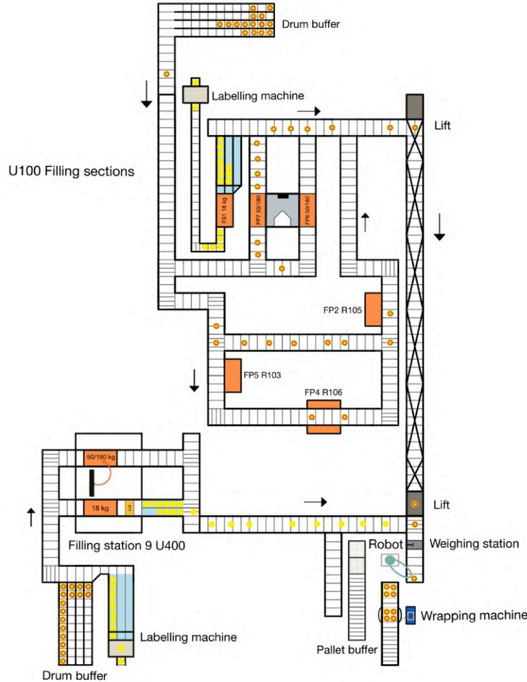
Figure 2.2: Schematic overview of EOL-section. Orange blocks correspond with the filling stations. Yellow dots represent 18 kg pails where yellow/red dots represent 50 or 180 kg drums.
