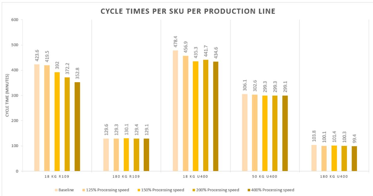
Figure 5.2: Results of the average cycle times per experiment 1-4 for the different SKUs filled at production lines R109 and U400
