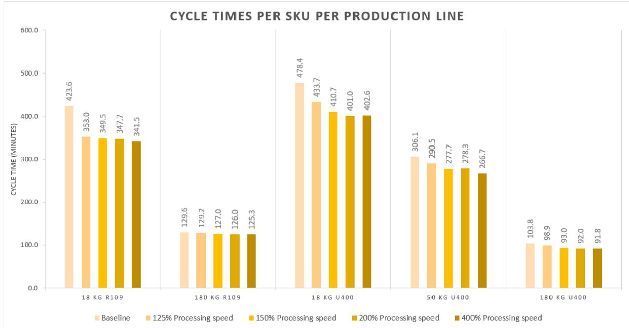
Figure 5.4: Results of the average cycle times per experiment 5-8 for the different SKUs filled at production lines R109 and U400
