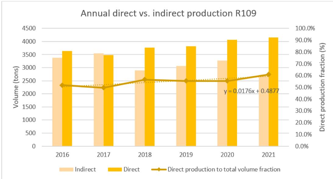
Figure H1: Overview of the annual production of both direct and indirect batches for production line R109. The trend line confirms the upwards trend in the production of direct batches on R109 over the past five years.
