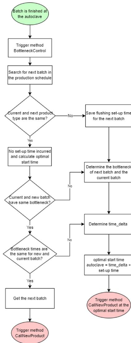
Figure 4.3: Flowchart of the bottleneck control mechanism in the production process. This logic holds for both the R109 and the U400 production lines.
