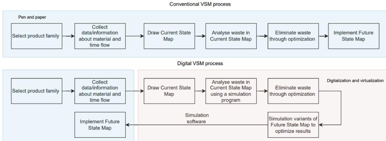
Figure 3.4: Overview of the differences in approaches between the traditional VSM and the combination of simulation modelling and VSM. (Esfandyari et al., 2011)
