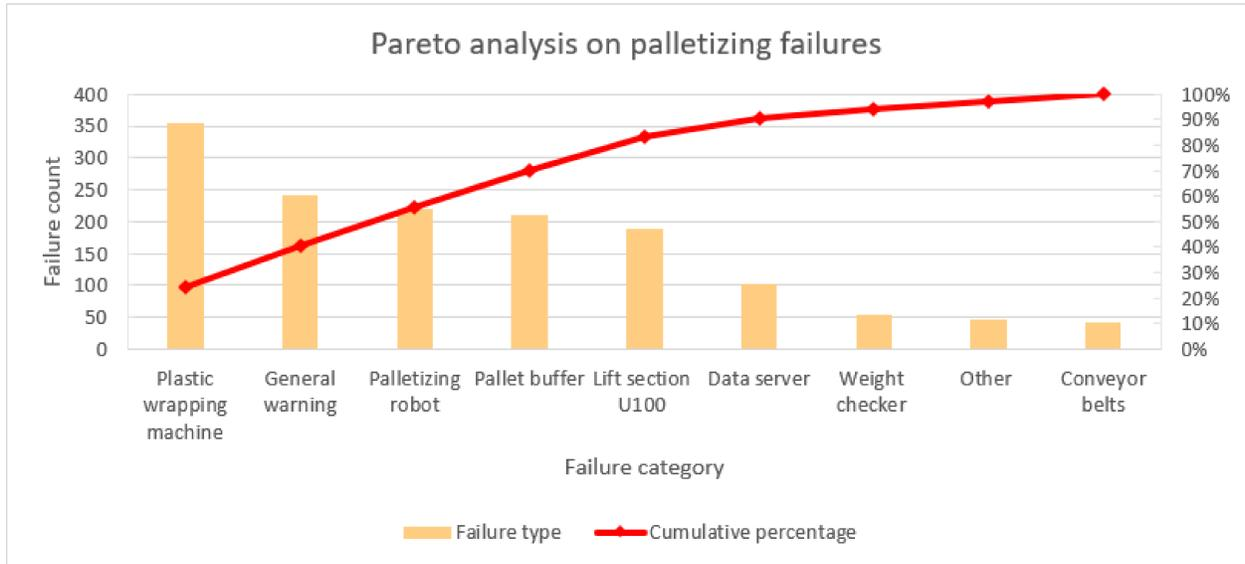
Figure 2.4: Pareto analysis of the failure categories and failure counts for the systems and processing units surrounding the palletizing robot
