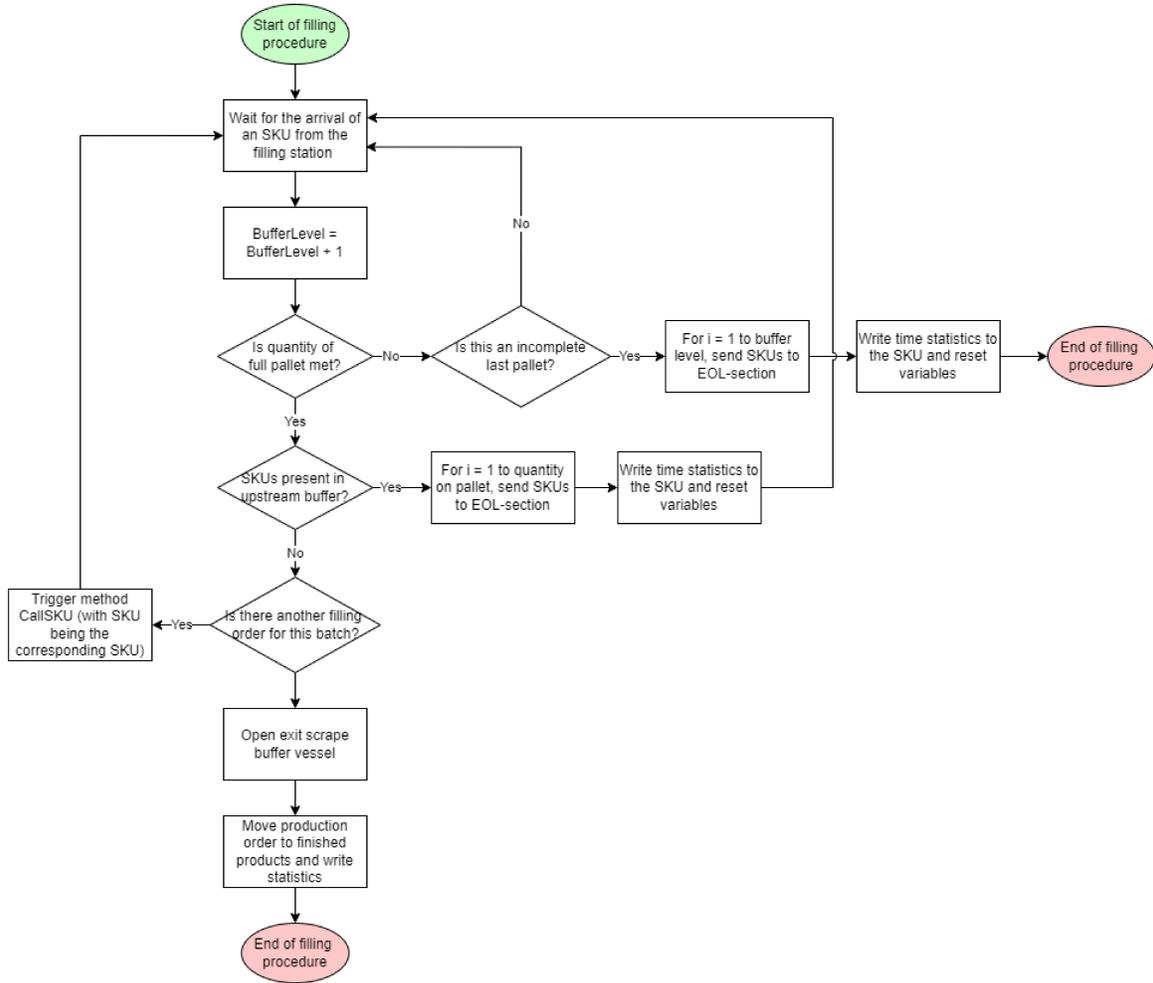
Figure 4.6: Flowchart for the buffer control mechanism that allows to move all the filled units to the EOL-section. This is dependent on whether or not a full pallet or the last pallet have been produced. For the U400, we simultaneously stop the filling station whenever a full pallet is being moved to the EOL-section.
