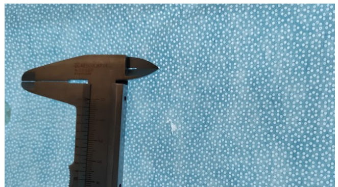
Figure 45: Tear found in sterile wrap after functionality test, caliper for size reference
