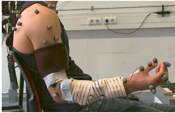
Figure 1: Placement of the passive reflective markers on the subject.
