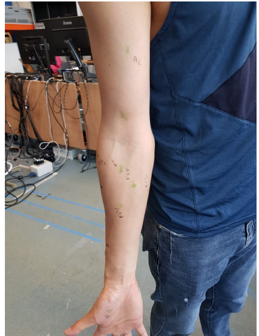
Figure 11: Muscle positions for EMG surface electrodes marked with a pen.
