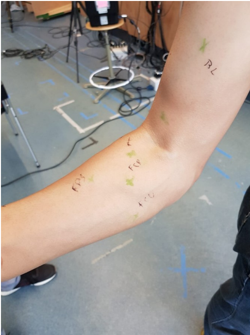
Figure 11: Muscle positions for EMG surface electrodes marked with a pen.
