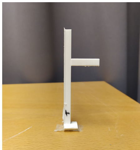
Figure C.1: Support structure for the placement of 3 markers on each hand segment
