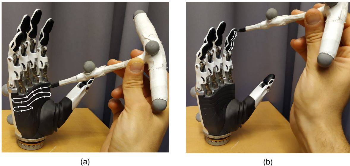
Figure 3.7: (a) Probing of the palm surface the white line shows an example of the path followed during the probing. (b) Probing of the finger surfaces, the white line shows an example of the path followed during the probing.
