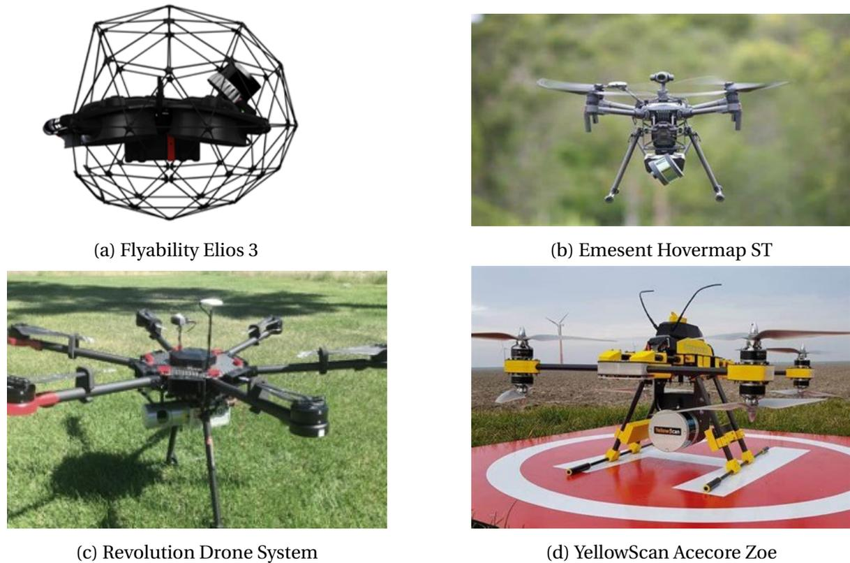
Figure 2.2: Mobile Mapping Aerial Platforms
