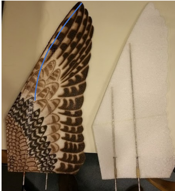
Figure 2: Finished (left) and unfinished (right) RoBird wing. The blue line indicates the position of the carbon fiber reinforcement strip. Modified from [Groot Koerkamp, 2018]
