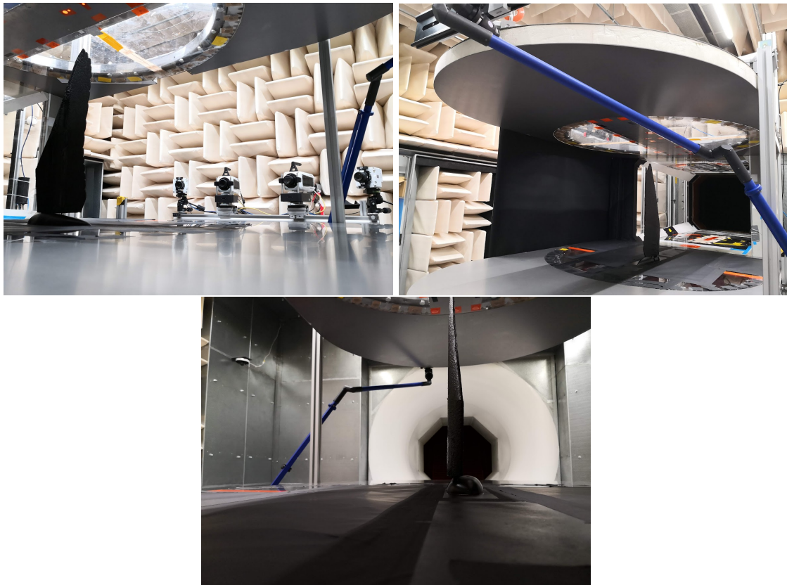
Figure 52: Measurement set-up for measuring the flow over the top of the wing
