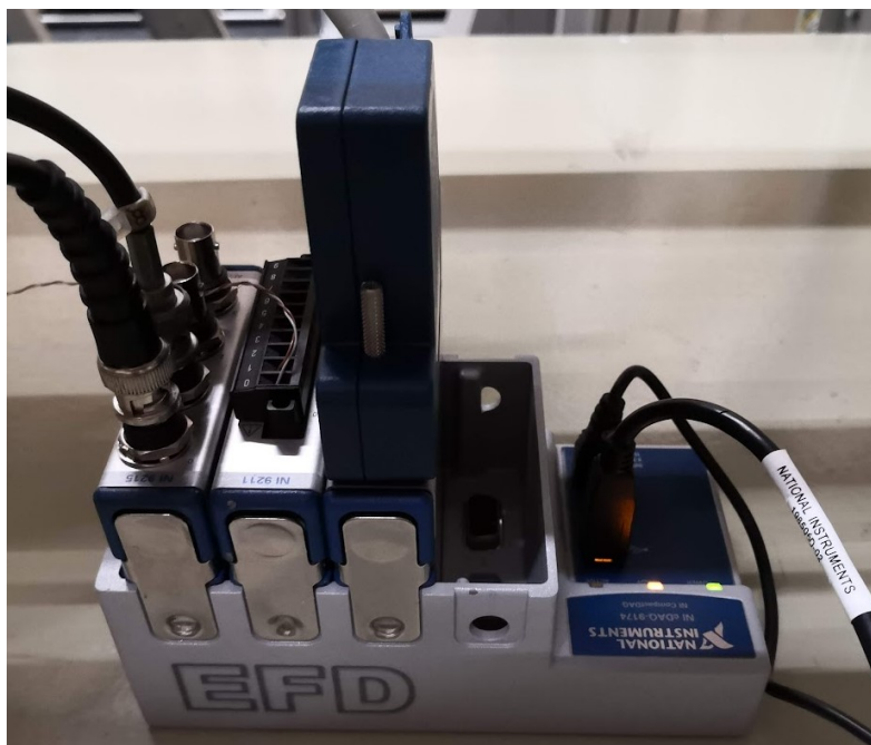
Figure 25: Data Acquisition System for force measurements
