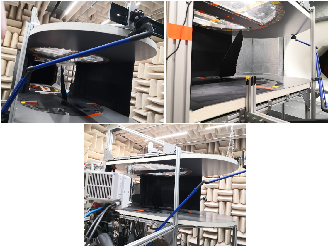
Figure 51: Measurement set-up for measuring the flow over the bottom of the wing
