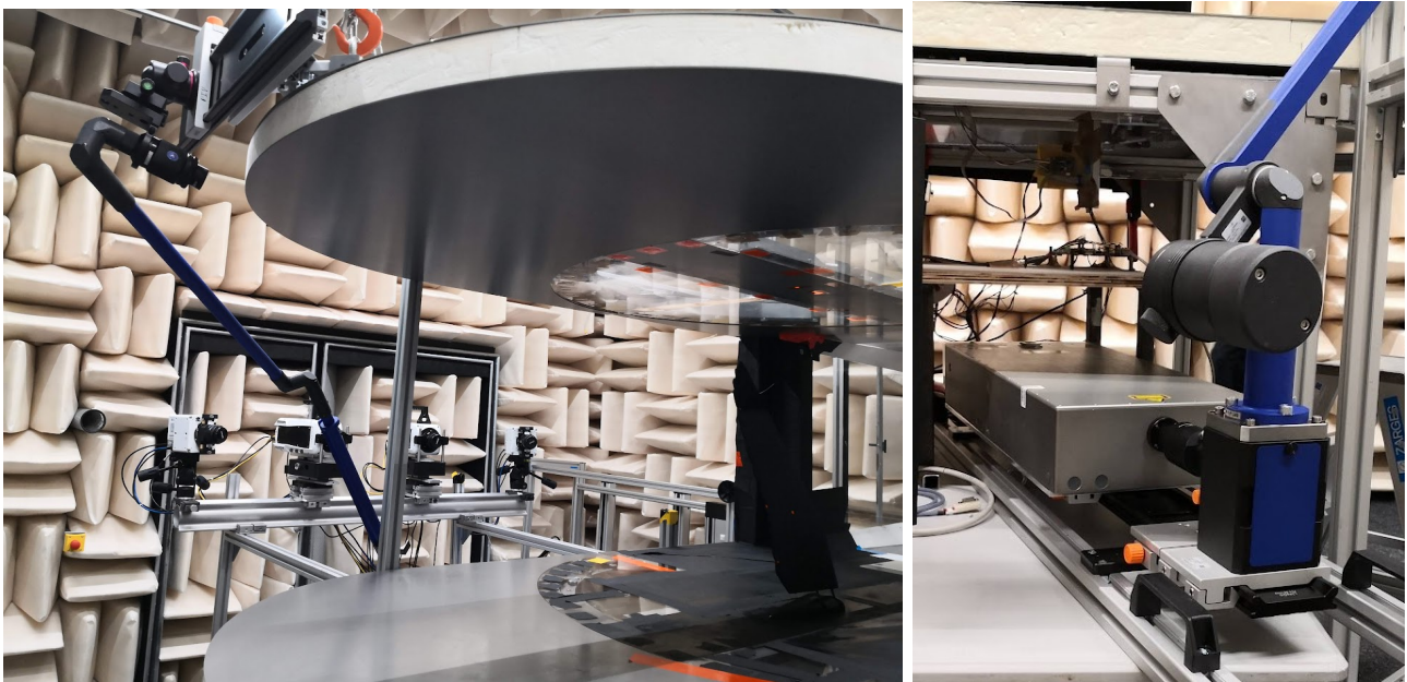
(a) Four high-speed camera's mounted on a stand and laser guiding arm (b) Laser connection with laser guiding arm mounted on top of the semi-open test section all directed towards the arm bottom of the wing
