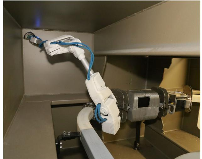
Figure 11: Proof of principle robot-arm, with covers, mounted on the drive unit. The relative pose of base- and end-effector is similar to the relative pose of  $\Psi_B$  and  $\Psi_3$  from fig. 3.
