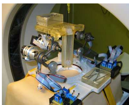
Figure 2.4: The prototype of the CT-Bot by Maurin et al. [5].
