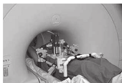
(b) The LPR placed on top of a patient in right outside an MRI bore.
