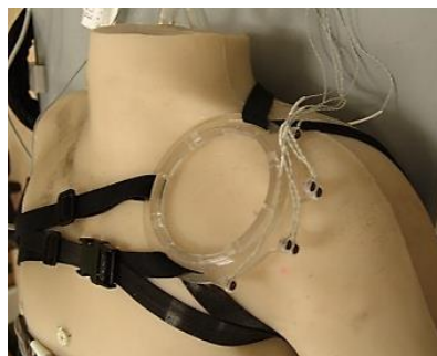
Figure 2.3: Fixation method using straps and a disposable adaptor for a shoulder-mounted robot [4].
