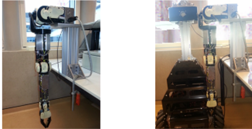
Figure 1.1: The Philips robotic arm (left) and the platform and body of the Bobbie robot (right)
