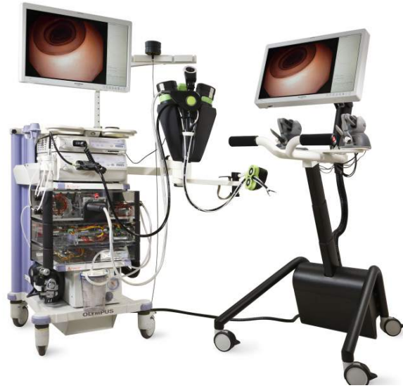
Figure 1.5: An overview of the TeleFLEX system (from Demcon 49 ). To the left the endoscopy stack can be seen with the video processor, light generator, and the actuators for the endoscope and instruments. To the right, the telesurgical workstation can be seen.
