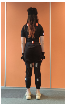
(a) A subject with 17 IMUs on different body segments.
