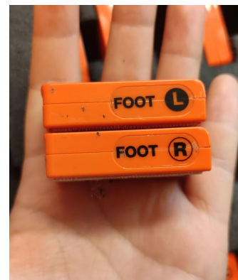
(c) Each IMU has a sticker on it to indicate the respective segment.
