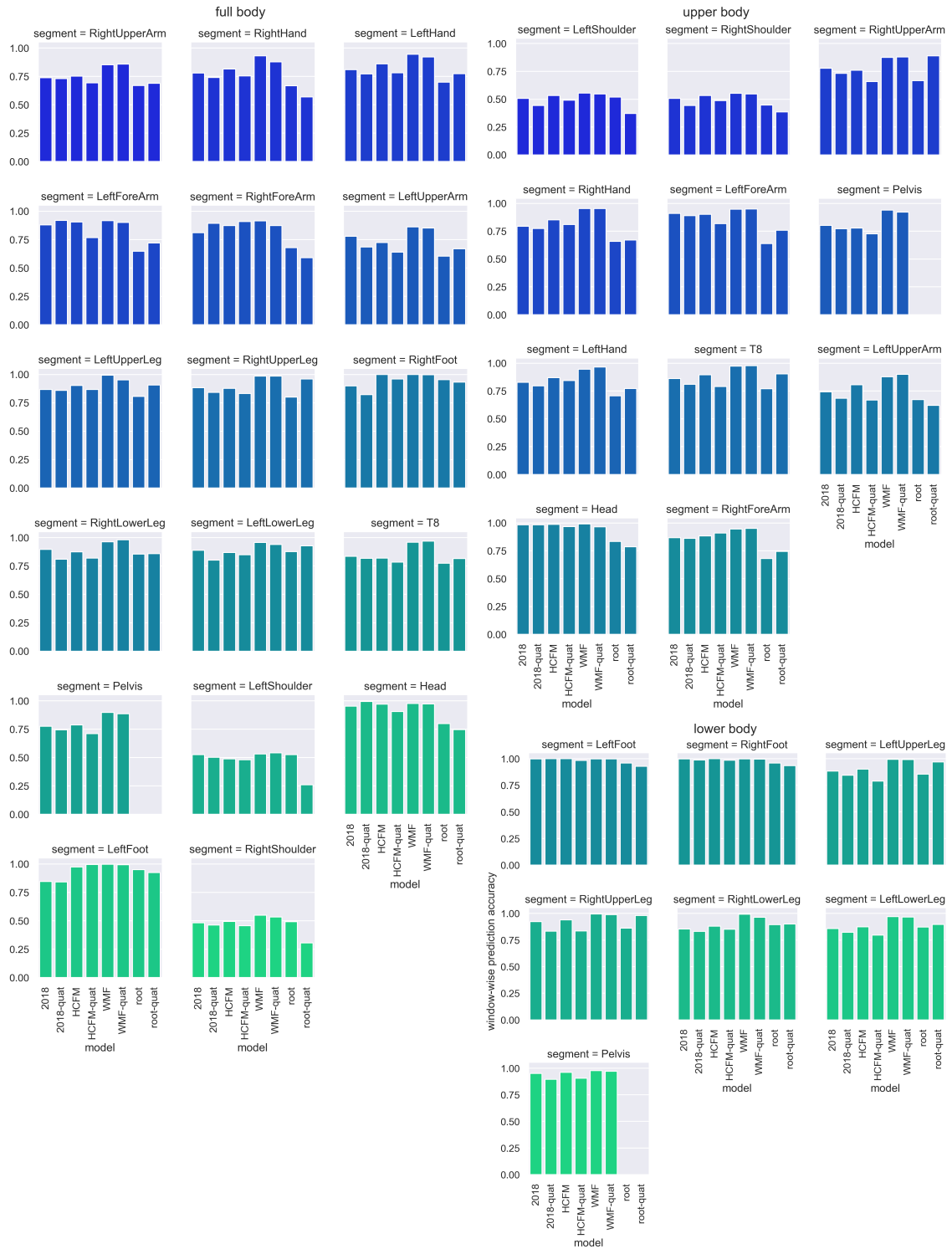
Figure 4.5: Bar plots of accuracy(y-axis)-model(x-axis) relationship. Model names can be found at the bottom under x-axes. The names include "quat" represent 10-channel input, "WMF" for HCFM with WMF (Exp.3) and "root" for HCFM with heading correction (Exp.4).
