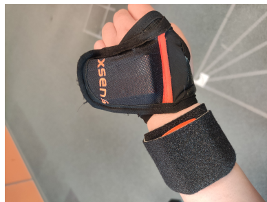
(b) The wrist and strap used to attach the IMUs to the body.
