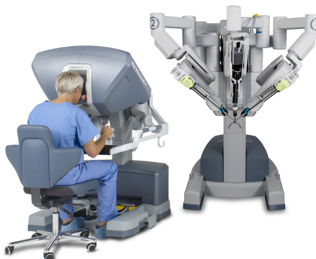
Figure 2.8: The Da Vinci surgical robotic system with human interface and robotic system. [23].
