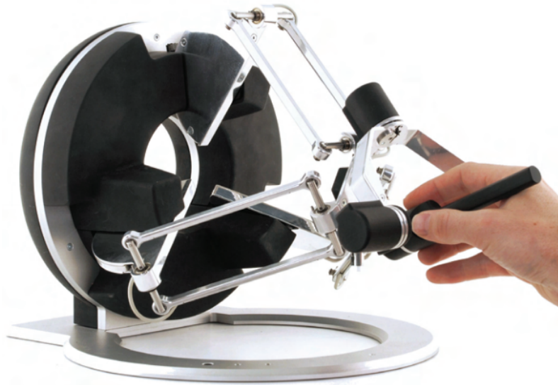
Figure 2.1: The Omega 6 haptic joystick with 6 degrees of freedom [4].
