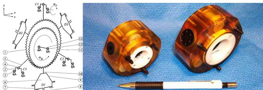
Figure 2. 10 Left: Kinematic diagram of PneuStep motor by Dan Stoianovici et al. Right: Two sizes of the motor prototypes.[17][18]
