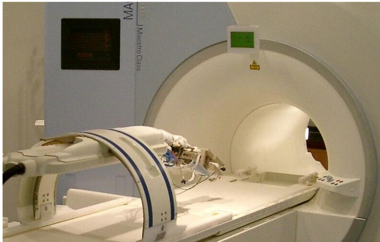
Figure 2. 7 InnoMotion robotic assistance system on the patient table of a clinical 1.5T whole body MR system.[14]
