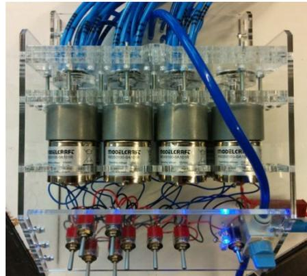
Figure 4. 3 The pneumatic distribution system.[47]
