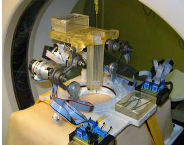
Figure 2. 6 CT-Bot prototype by Benjamin Maurin et al. with a passive needle guide.[12]
