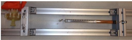
Figure 10 Output force measurement instrument for actuator.
