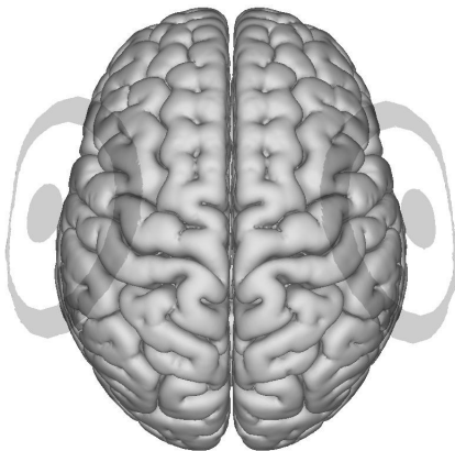
Figure 3: The general set-up of the center-surround ring electrodes. The inside electrode of the rings is placed on C3 and C4 EEG electrode positions. The exact diameter of both the inside and outside electrodes will be varied in simulations.
