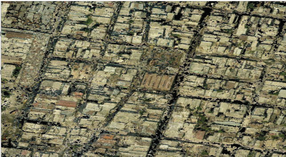
Figure 3-2. Aerial Oblique Photograph generated point cloud visualized using own colour.
