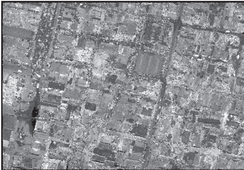
Figure 3-1. LiDAR point cloud visualized using reflectance.
