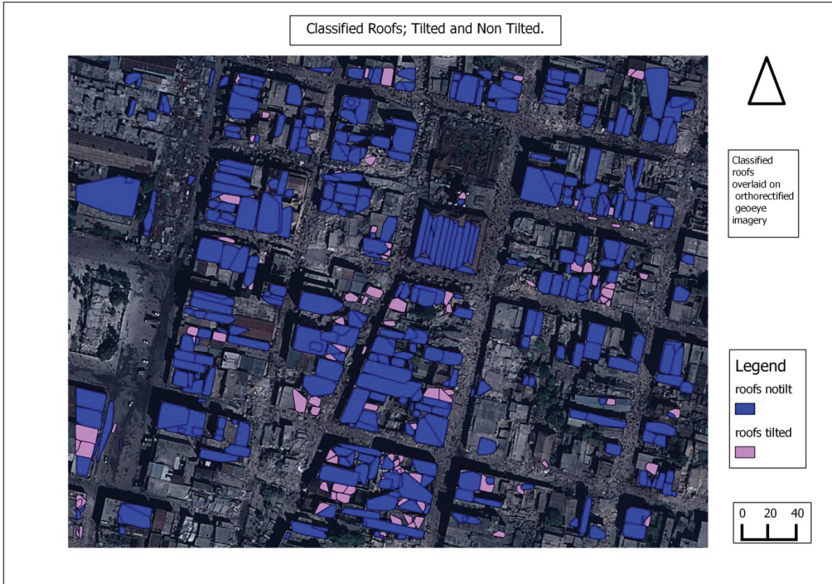
Figure 6-9. Roofs, Tilted and Non Tilted
