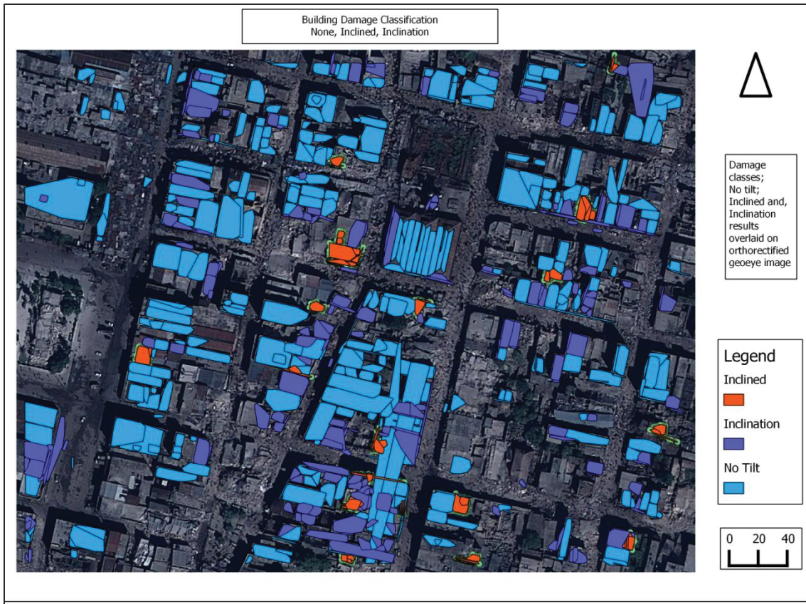
Figure 6-7. No Tilt, Inclined and Inclination damage classes
