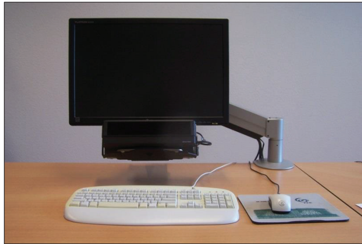
Figure 4-1: The eye tracking system in the desktop setting
