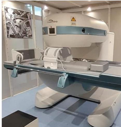
Figure 6: Picture of the 0.25T full body scanner, which is also able to perform upright acquisitions.
