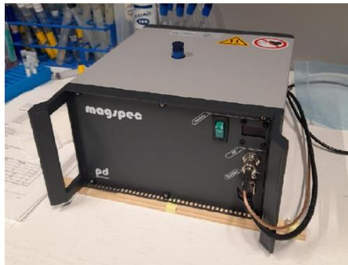
Figure 4: Picture of the 0.5T tabletop scanner.
