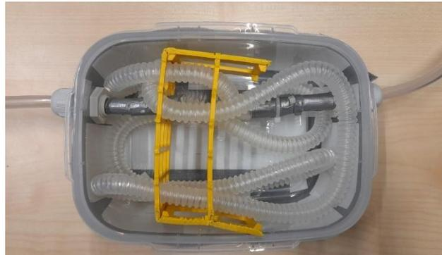
*Figure 8: Picture of the isolated box used in the heat regulation setup. Through the internal pipesystem 39°C water is run through which keeps the water inside the box at 37°C. Samples tubes can be placed inside the yellow brackets.*
