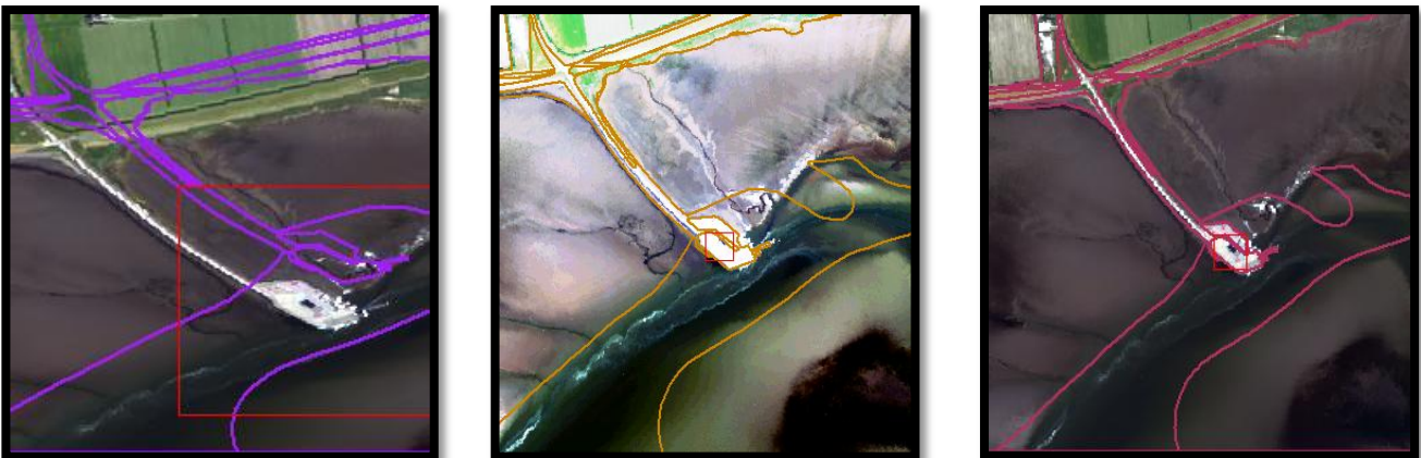
Vector overlay showing harbor of Schiermonnikoog. Emphasis on building (dark pixels) position relative to vector overlay.
