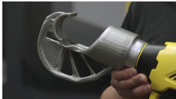
Figure 1.4. A 3D-printed clamp, topologically optimized in Autodesk [24].
