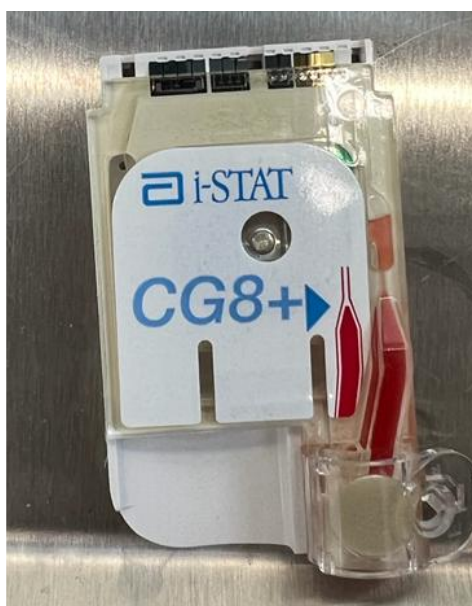
Figure 18: Left: i-STAT Alinity device for blood measurements. Right: CG8+ cartridge for measuring blood parameters. The cartridge is filled with blood and inserted in the device, which will read out values after several minutes. The table presents the parameters that are measured using this cartridge.
