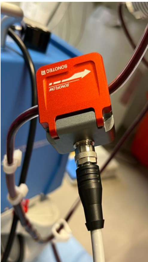
Figure 7: Sonotec flow sensor clamped onto 1/8" tubing for flow measurements.
