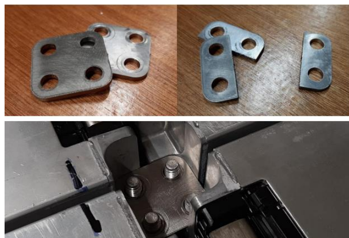
Figure 29: Cookies used to reduce the flexibility
