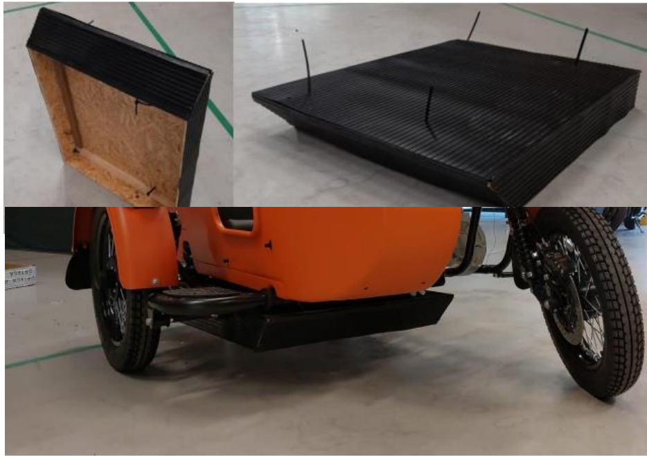
Figure 24: Wooden mock-up of the battery case
