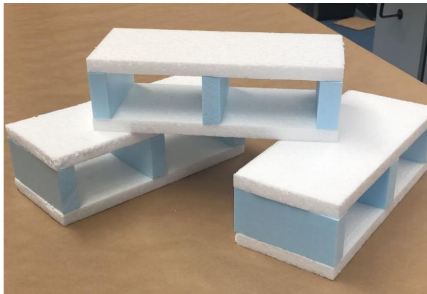
Figure 22: Foam duplicates of the battery modules
