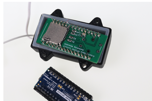
(b) Back side, this side has the SD-card reader as well as the header pins to connect the shield to the Arduino.
