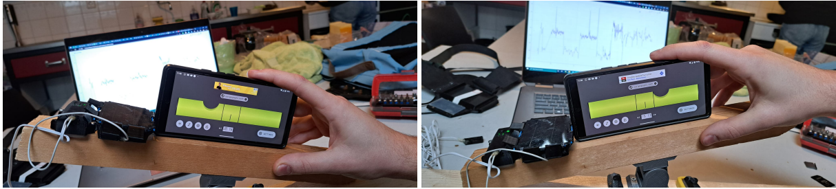
(a) Setup tilted to the far right. Using phone app for angle reference, value on screen shows 20.16^\circ . (b) Setup tilted to the far left. Using phone app for angle reference, value on screen shows 15.13^\circ .
