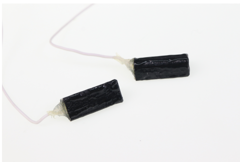
(a) Sealed vibration motors in a 3D print and epoxy glue.
