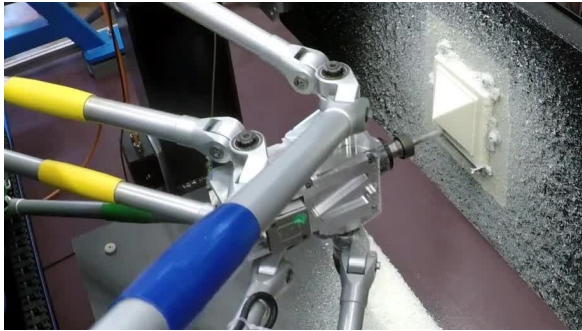
Figure 2.1: Milling of a pyramid using a pre-planned path, video still adapted from [8].
