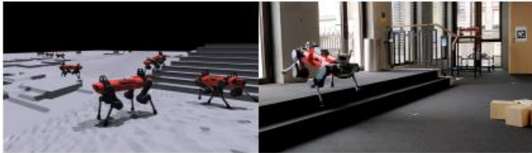
Figure 7. The difference between simulation and real-world application. The left picture shows training in a simulated environment. The right picture shows testing of the policy in the real world. Without simulation software, the training is in the real world, increasing the possibility to damage the robot, environment, or both (Makoviychuk et al., 2021).
