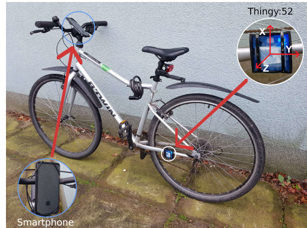
Figure 1: Bicycle System with Thingy Sensor and Phone
