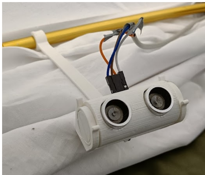
Figure 19: Sensor in 3D-printed mount
