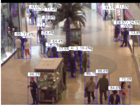
Fig. 6. YOLOv7-tiny result with Gaussian Blur r = 1\text{px}
