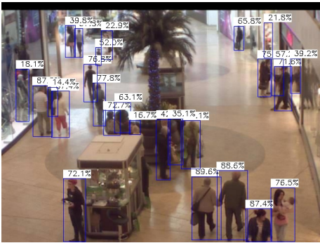
Fig. 16. YOLOv7-tiny result with "Lens Blur" r = 4\text{px}
