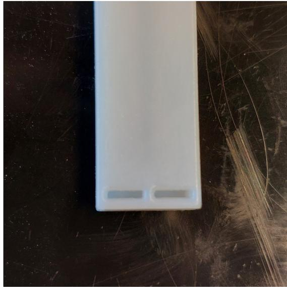
**Figure A.3:** Slit in inner tube of prototype 4 printed out of VeroWhite using the Connex3
