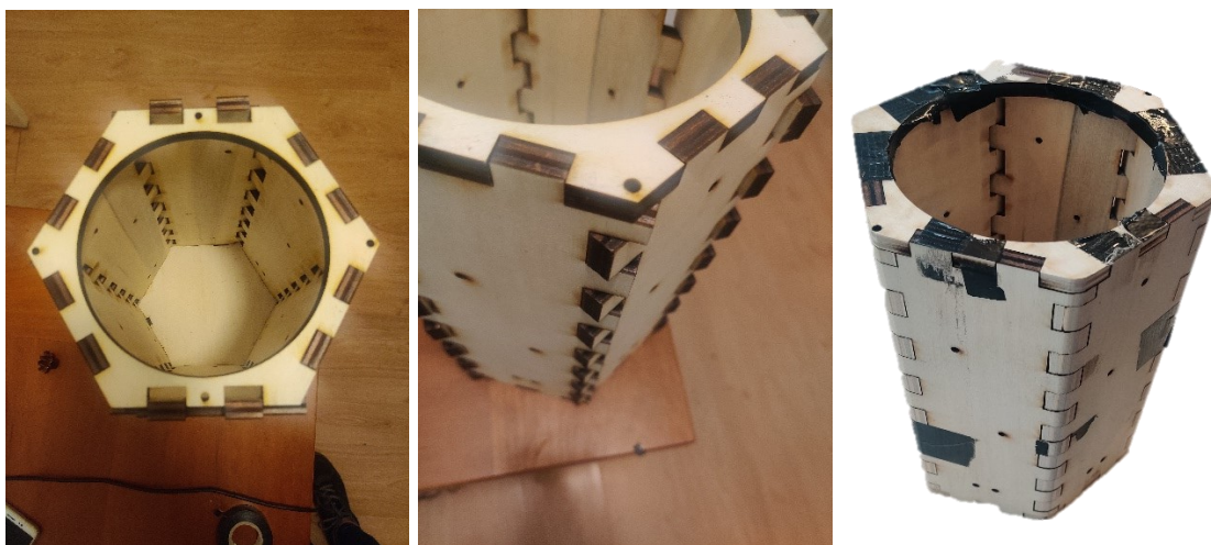
Figure 75: External box. Left to right: (a) top view (b) finger joints (c) smooth corners
