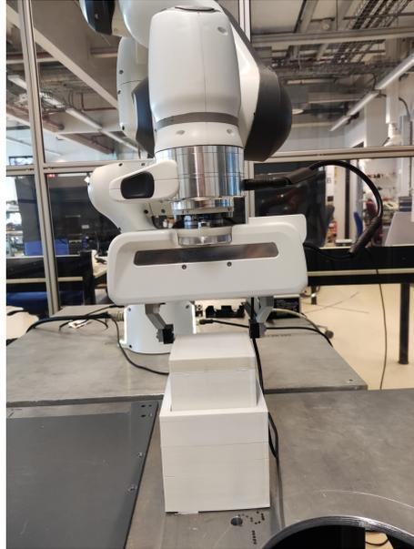
**Figure 6.1:** Setup of the Robot Franka Emika with the F/T sensor ATI Mini40. The force sensor is placed between the robot and the panda gripper
