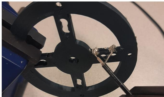
**Figure 3.10:** Silver epoxy connection for the attachment of wires to the strain gauges of an early iteration of the sensor.
