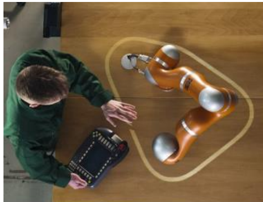
Figure 14 Dynamic safety zone established around the cobot [38]
