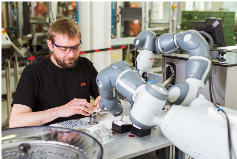
Figure 1 YuMi (a product of ABB) working together with a human for socket assembly [9]
