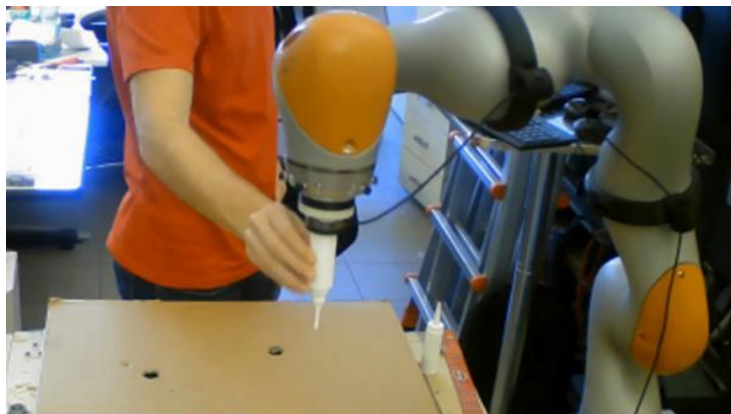
Figure 13 Experimental setup for hand guiding [36]
