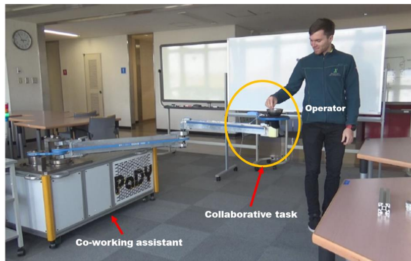
Figure 19 Experimental setup for motion planning with PaDY[44]
