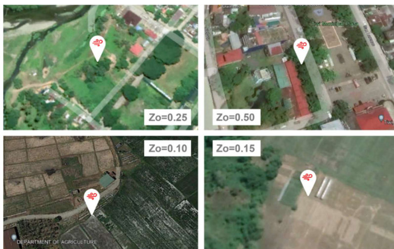
Figure 29 Example of four imagery with locations of wind observation stations, and the corresponding roughness coefficient ( Z_o ) assigned to it
