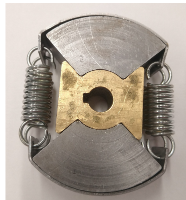
Figure 4.2: Centrifugal brake with new brake linings
