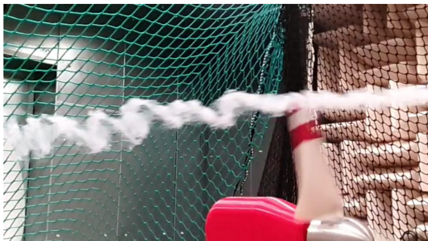
Figure 7.14: Tip vortex creating observed from smoke inserted into wind
