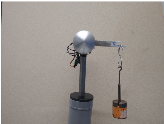
Figure 6.2: Torque calibration front view
