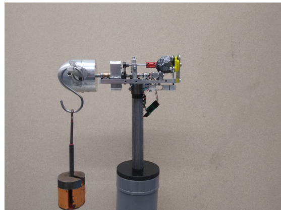
Figure 6.3: torque calibration side view
