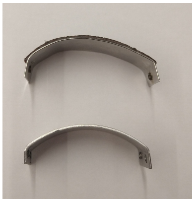
Figure 4.1: Old brake lining (upper) and new brake lining (bottom)
