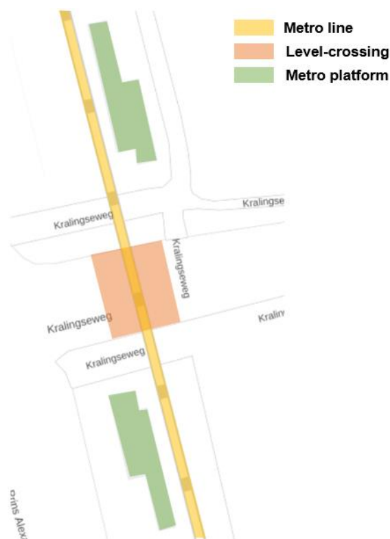
Figure 3: Example of level-crossing with staggered platforms
