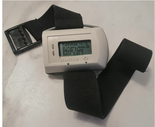
(c) The PuppyNose with a hydrophobic mesh and without a washer under it. This design resulted in a sensor malfunction.
