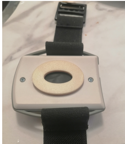
(c) The backside of the PuppyNose. A mesh covers the opening and an elliptical cushion seals off the skin and forming a semi-closed chamber.
