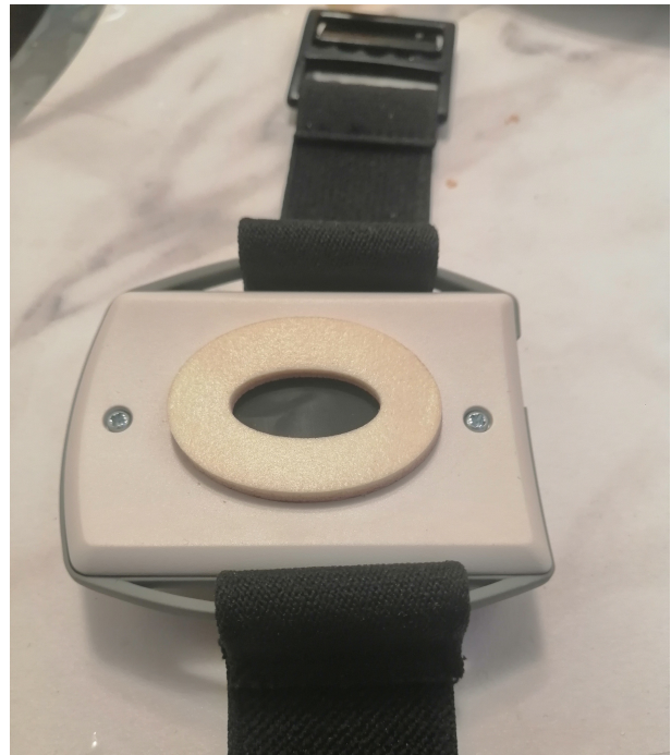
(d) The final design with the HD10BHY hydrophobic mesh and the elliptical cushion to seal of the skin.
