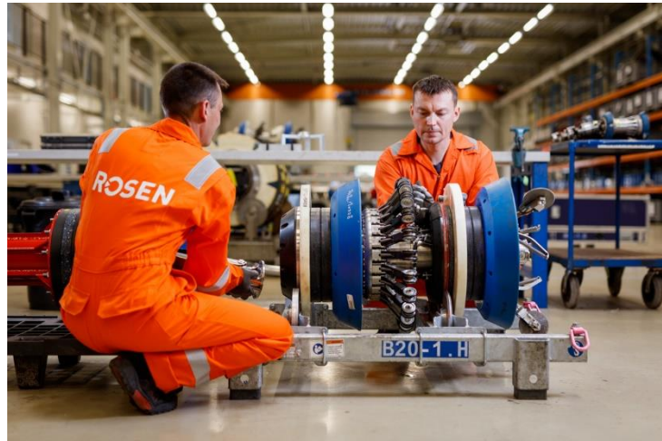
Figure 2: Work on an in-line inspection tool, with the holding frame and plastic accessories also visible (ROSEN Group, 2020)
