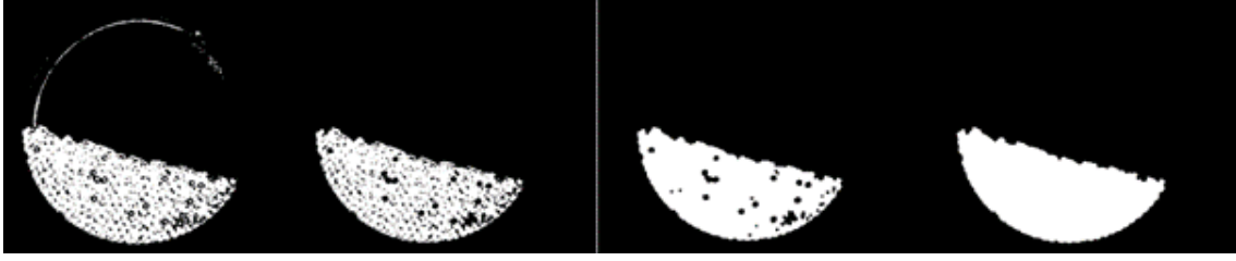
Figure 16: a)Black white particle segment b) close small object c) close small segments d) close holes
