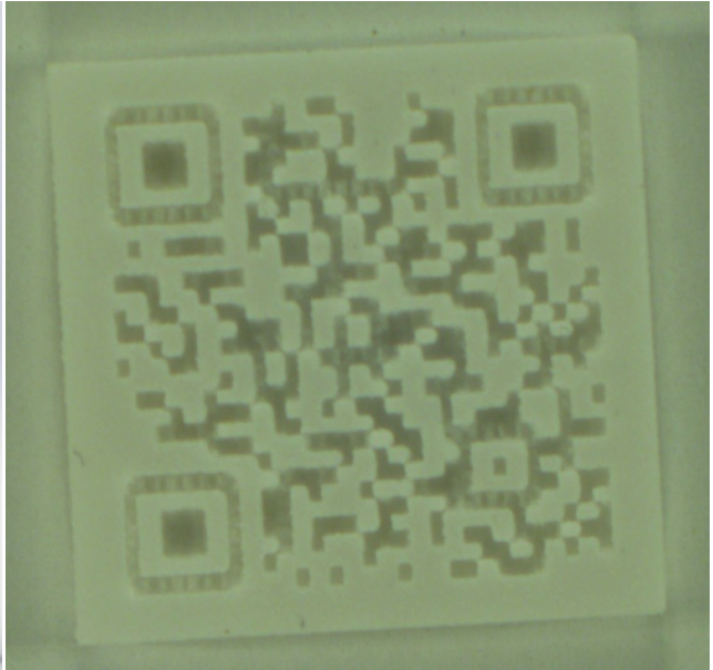
Figure 6.7: A render of a QR code with a circle Figure 6.8: An example of a sample with a pattern (C0.2) and a carving depth of 0.8 mm.
