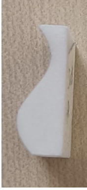
Figure 6.21: The ACsinP1A3 sample, with a period of 1 and an amplitude of 3.
