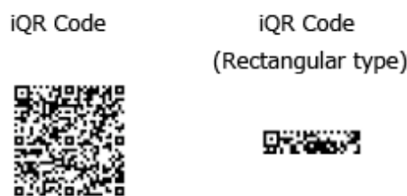
Figure 2.14: A normal (left) and a rectangular iQR code.
