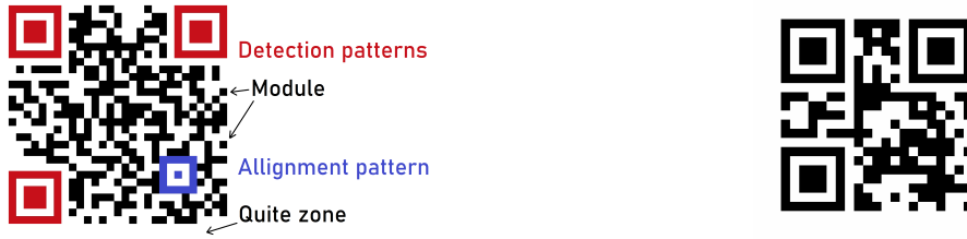
Figure 2.11: An example of a type 2 QR code. Figure 2.12: An example of a type 1 QR code.
