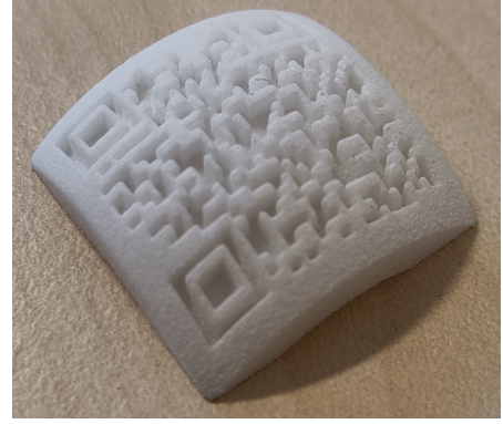
Figure 6.23: The ACD3030 sample with a curvature in two directions.
