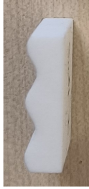
Figure 6.22: The ACsinP2A1 sample, with a period of 2 and an amplitude of 1.
