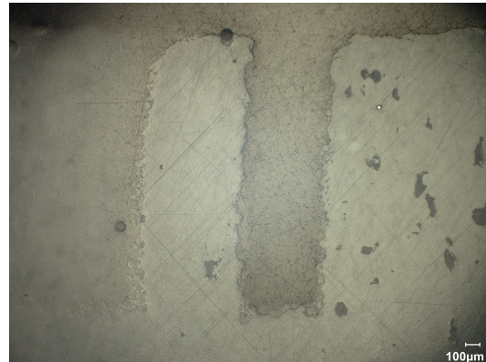
Figure 8.10: A hole with a width of one module in the size 19 mm sample without at the bottom of the negative module.
