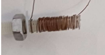
Figure 23: Photo of the coil used in testing. The coil is made using a wire with the diameter of 0.0001 mm which is wound 36 times around a plastic screw with a diameter of 3mm.
